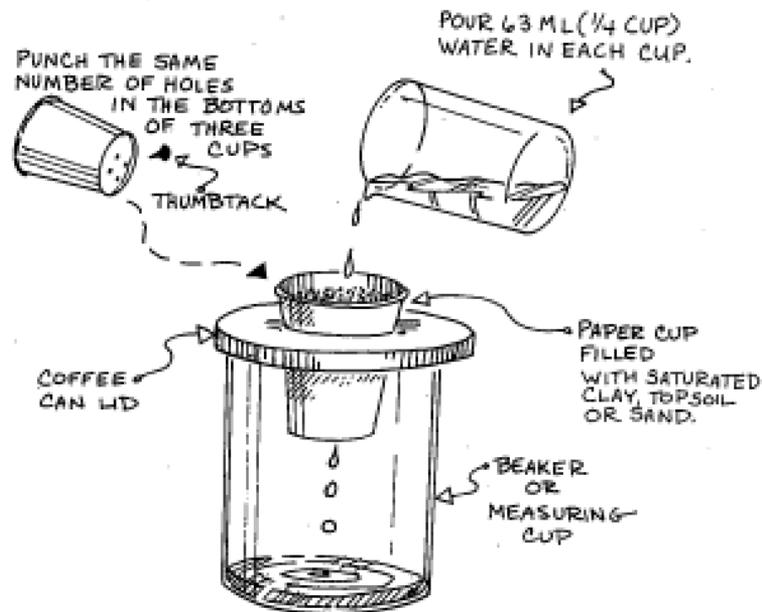
3. Pour 1/4 cup (63 mL) of water into the first cup. Have the students record the time when the water was poured.
