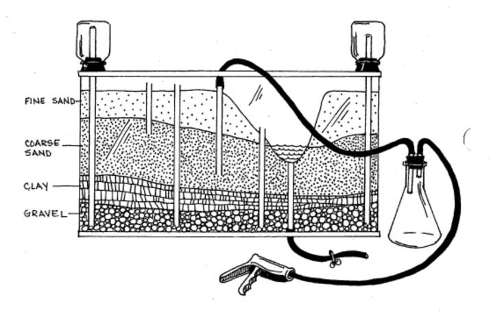
This groundwater model is a very effective tool for demonstrating the hydrogeologic cycle, for showing the effects of well pumping, and for showing how human activities can contaminate
