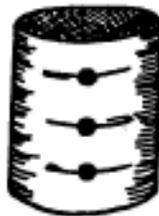
2. Have students hold a ruler out beside each hole. Simultaneously remove the plugs and allow the water to spray into the dish pan. Measure the greatest projection from each hole.
